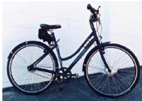
*A pedelec is a type of e-bike or power-assisted bicycle that has working pedals and a small electric motor that is triggered while the rider is pedalling, reaching a maximum speed of 25km/h during assisted pedalling and weighing less than 40 kilograms.*
